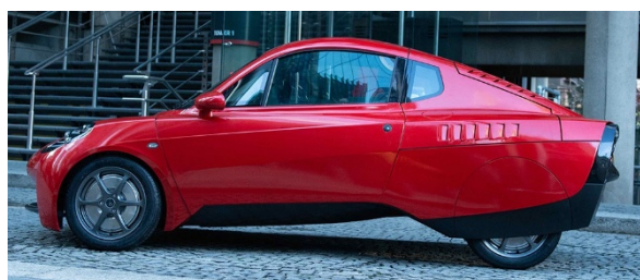
Figure 13: The Riversimple Rasa, small hydrogen fuel cell car with a 300 mile range
